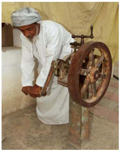
down to less than one millimetre through which wires are pulled. Drawn wires are typically recognisable under an optical microscope from their uniform diameter and the numerous fine parallel grooves clearly visible on the surface along their length. The various components are next assembled by extensive and meticulous silver brazing with a zinc- and copper-rich silver solder or mechanically as with loopin-loop wire chains and joining rings.
