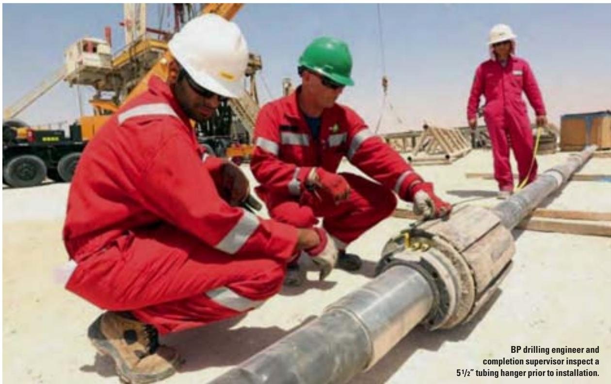
BP drilling engineer and completion supervisor inspect a 5 1/2" tubing hanger prior to installation.
